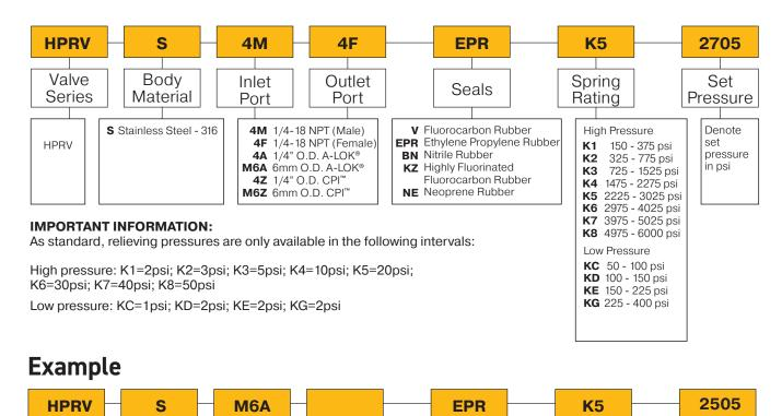
Describes a HPRV Series proportional relief valve equipped with 6mm A-LOK® compression inlet and outlet ports, ethylene propylene rubber seals, stainless steel construction, fitted with A 2225-3025 psi spring. Supplied pre-set at 2505 psi.
