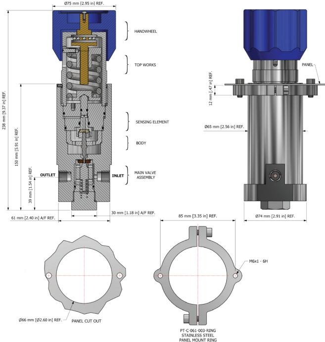
All gauge ports are 1/4" NPT as standard - max. 690 bar (10,000 psi) supply pressure on NPT - use MP for higher pressures.
