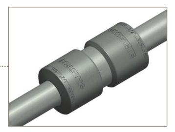
The tubes are simply inserted into the Phastite<sup>®</sup> connector, adequate tube insertion is assured by using the Phastite<sup>®</sup> tube marker.
